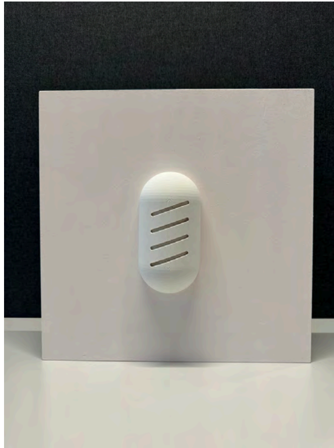
Image 22: 3D-printed shell on wooden ceiling tile
