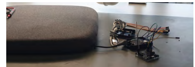
Figure 16. The sensor cushion and the electronics inside. A breakout board was temporarily soldered to the sensor chip, to upload the new firmware.
