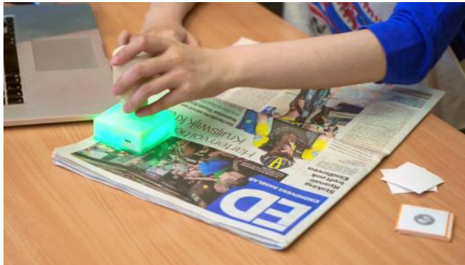
Figure 5-14 In the Edit Mode, caregivers can quickly add IStickers to R2S system by 'stamping'.
