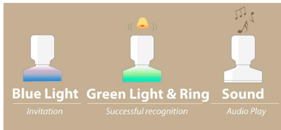
Figure 5-12 The visual and auditory feedback of IStamp are designed to facilitate older users.
