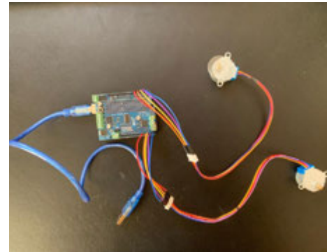
Figure 5.2.2.1 Connections of Steppers, Motor Shield, and Arduino Board
