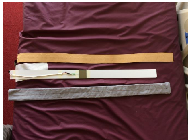
Figure 3. Top view of two piezoelectric sensors (first two strips from above) which have the length of the full width of the bed.
