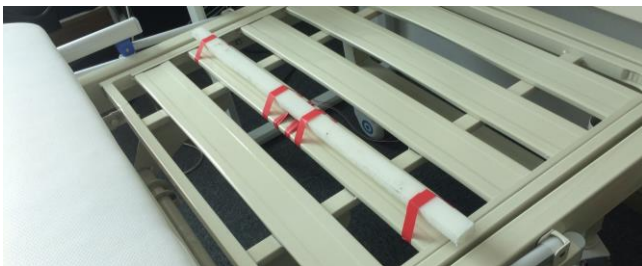
Figure 12. Load cell proof of concept prototype with POM bar on top to focus the force on the load cells.
