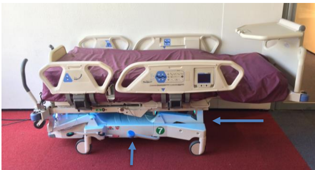
Figure 8. Hospital bed with interactive LED light below. In this case nobody is on the bed so the light is blue.
