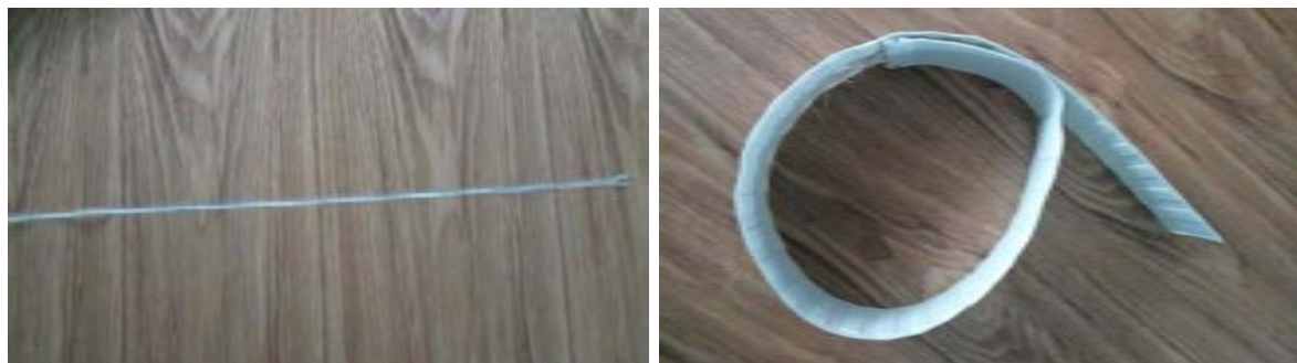
Figure 1. Left: Pressure sensor – Piezoelectric PVDF films Right: Belt containing the PVDF Piezoelectric films
