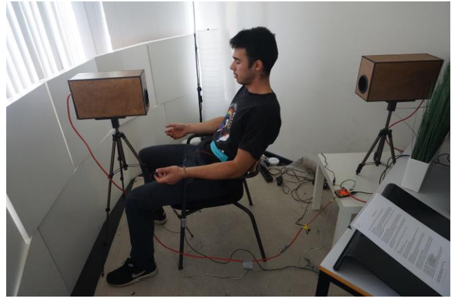
Figure 1. Setup: participant sitting between two air fans with equal distances, wearing a respiration belt and PPG sensor.
