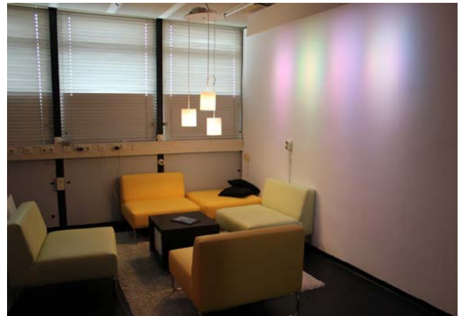
Figure 4. Test room setup with comfortable seats. Picture shows the side of the waiting room with incandescent lamps and full color LED wallwasher where participants were asked to wait.
