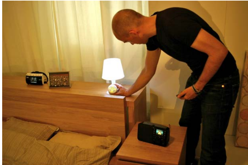
Figure 26: The sleep use case scenario, with the Zeo sleep monitor on the left, the dimmable light and the Connector object in the middle, and the Squeezebox on the right
