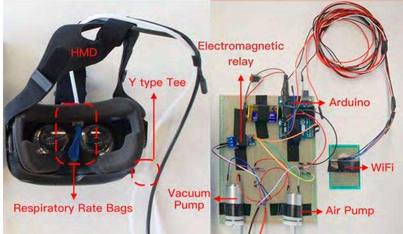
**Figure 4.** Respiration Simulator Details
