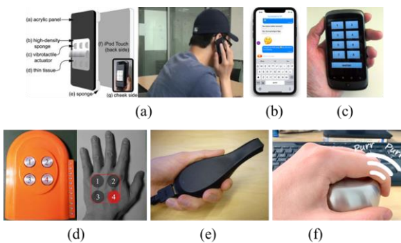
Figure 8. Typical examples of C1. (a) CheekTouch with attached actuators [10], [11]; (b) An iPhone with an embedded Taptic Engine for VibEmoji [71]; (c) The Google developer phone Nexus One with an embedded vibration actuator [82]; (d) PalmScape with four vibration actuators [84]; (e) a mouse-like haptic device with vibration actuators [1], [28], [29], [30], and [76]; (f) a handheld haptic device with a vibration actuator [26]; Figures are from the corresponding literature.
