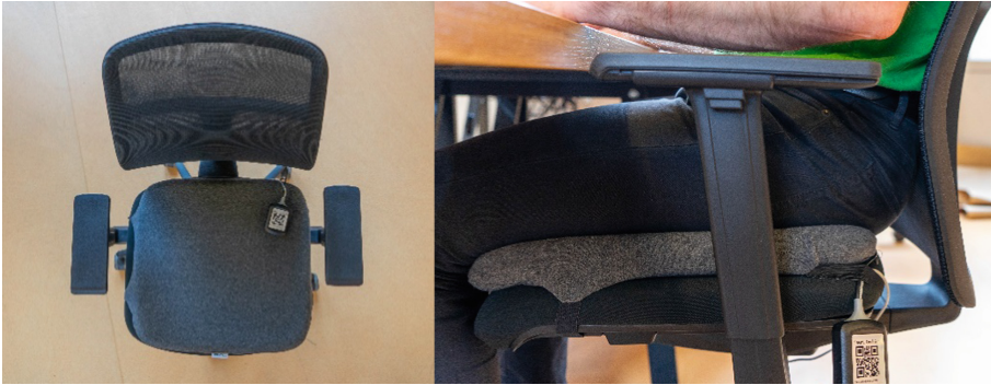
Fig. 1. Left - smart cushion on an office chair. Right - user working on the smart cushion (grey)
