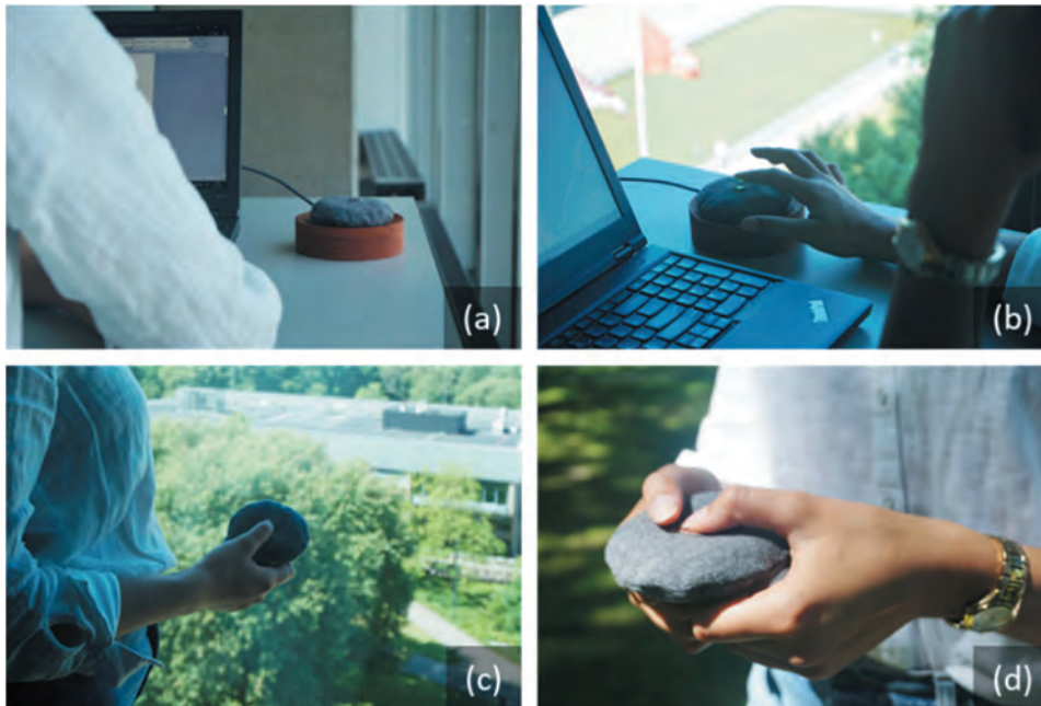
Figure 3. (a) The soft tangible interface of ViBreathe on its wireless charging dock placed on the desk within the user's reach; (b) the user can follow its haptic breathing guidance while simultaneously focusing on the computer screen; (c, d) the user can also hold ViBreathe to have "micro" relaxation training during a short break from work.
