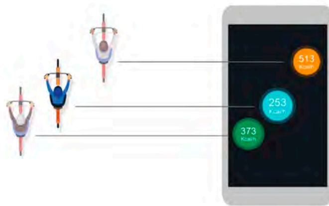
Figure 3. The position of the circle in the front display corresponds to the actual position of the cyclists (top view).
