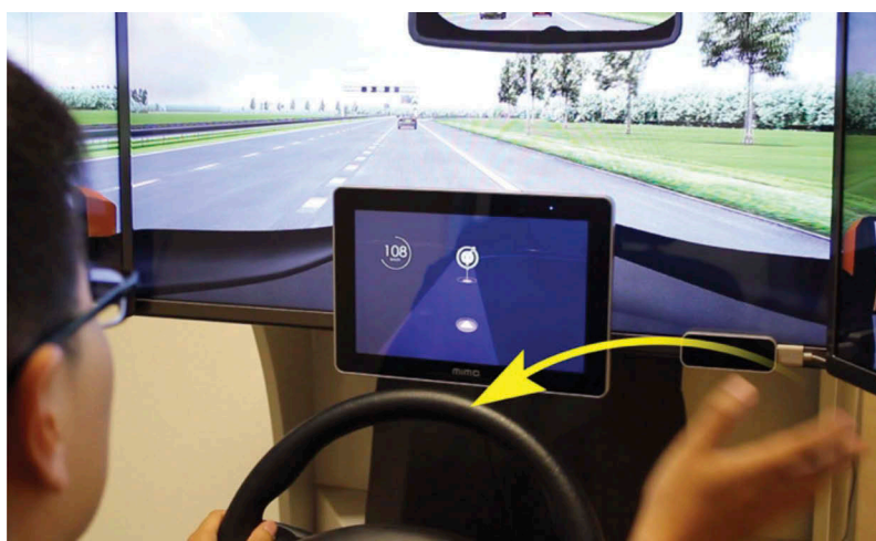
Figure 9. Wave hand in to “get” the music of other cars. The LeapMotion sensor is visible at the bottom right.
