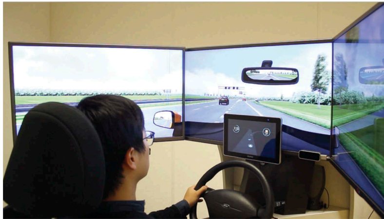
Figure 1. A 10" screen was integrated in the driving simulator.
