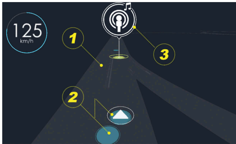
Figure 8. User interface design. 1) Geography layer; 2) Vehicle layer; 3) Notification layer.
