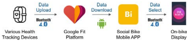
Figure 1. Schematic of SocialBike's technical system.
