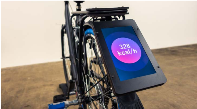
Figure 2. Prototype of SocialBike's on-bike display.
