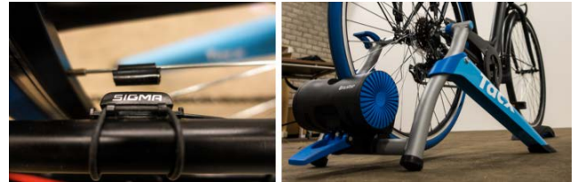
Figure 4. The reed switch and magnet used to detect the rotational speed of the bike wheel (left) and the bike trainer used to provide resistance (right).
