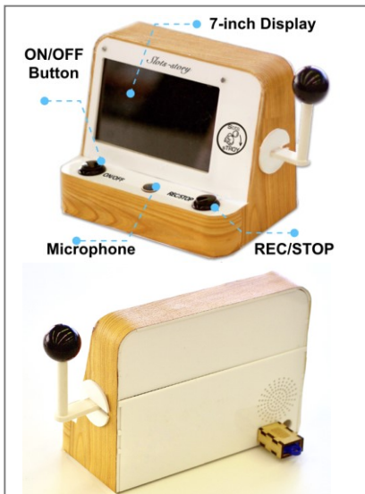
Figure 1: Its outlining shape is round-cornered, evoking an approachable and ergonomic design. Its L-shape makes the display easy to see, and buttons easy to access. Its portable dimension makes it easy to carry (L = 22cm, W = 11cm, H = 17cm). The main body is made of porcelain white acrylic, and part of it is covered with wood-grained paper, making it look slightly old-fashioned, which is in line with the aesthetic taste of older adults.
