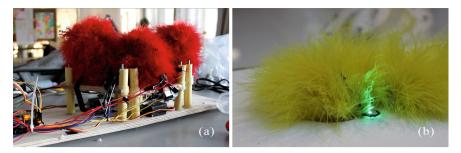
**Fig. 2.** The design details of *Dynamorph*. (a) Zoomorphic shapes consisting of three separate balls are mounted individually on mechanisms underneath the table to be programmed to respond correspondingly to user's gestures. (b) A zoomorphic shape powered by the interactive ball set with a pulse sensor embedded in the table.
