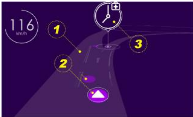
Figure 5: User interface design. 1) Geography layer; 2) Vehicle layer; 3) Notification layer
