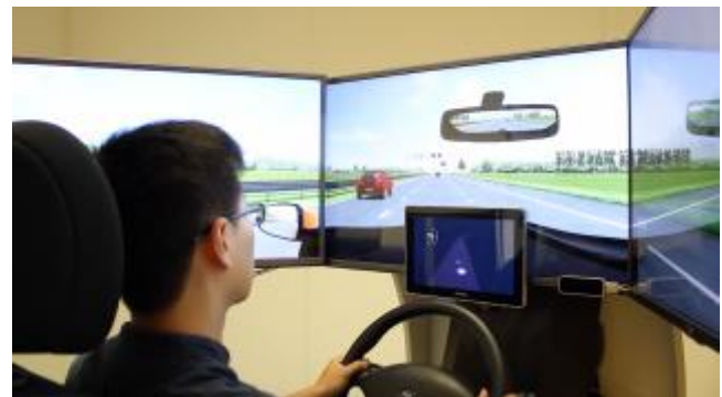
Figure 4. A 10" screen was fixed on the driving simulator.
