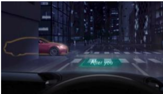
Figure 3. Lexus LF-FC concept car enable driver to send pre-set message by gesture, such as “After you” and “Thanks”, to nearby drivers.
