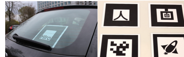
Figure 3: Each driver will have an unique AR marker as ID (later might be replaced by license plates).
