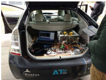
Figure 2 d-SPACE was implemented in the back of car.
