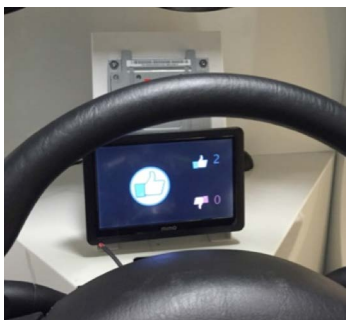
Figure 2: An 8" screen was set in front of the steering wheel to show other driver's evaluation.
