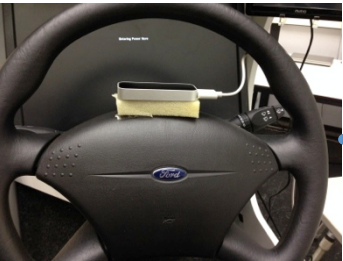
Leap motion fixed on the steering wheel
