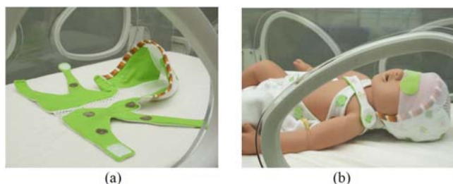
Figure 1 (a) Prototype smart neonatal jacket and (b) a baby mannequin wearing the smart jacket inside the incubator (see online version for colours)
