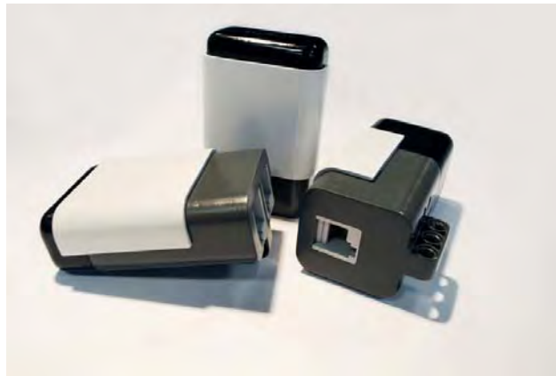
Fig. 3. The sender and receiver extensions for Lego NXT. The sender module has two inputs for two different inputs.
