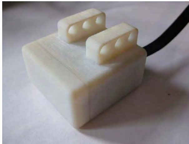
Fig. 4. The sensor casing with optical mouse sensor, the micro controller is not integrated in the casing yet.
