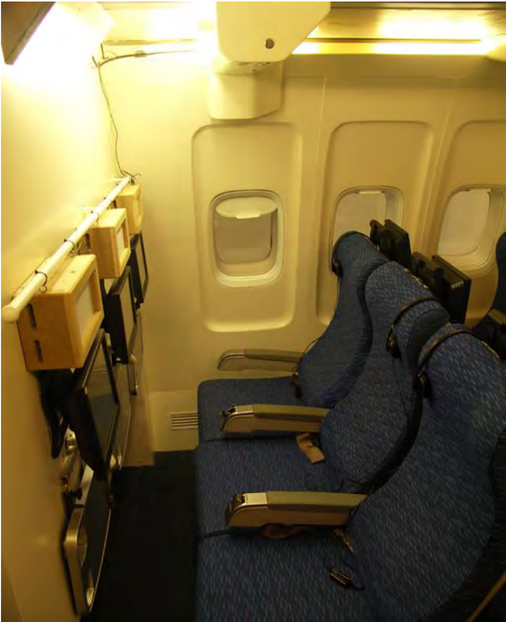
Figure 6.12, cabin lighting units placed in the simulation lab
