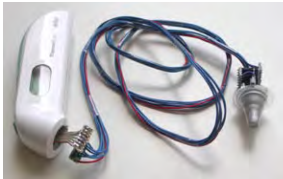
Figure 4.8, photo of adapted in-ear thermometer used to investigate the option to use this type of measurement to retrieve a human core body temperature curve.
