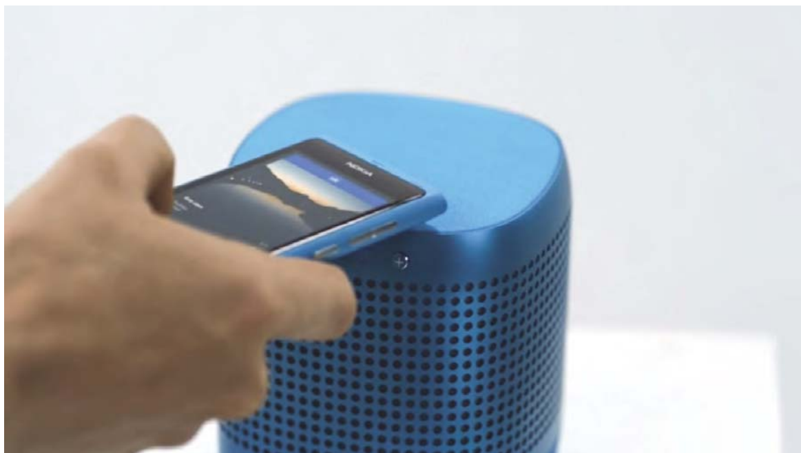
Figure 2.3: A user pairing an NFC enabled smart phone with the Nokia 360° speaker [image source: screenshot taken from advertisement video, available from: http://nokia.ly/ingpDX ]
