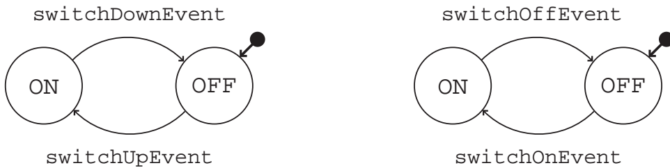
Figure 5.4: FSMs for a simple light with a switch and a light with a labelled switch
