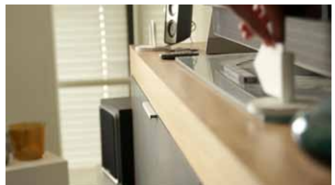
Figure 3 - The Nodes design being used: A user makes a connection between two Nodes by aligning the sender (starting point of a connection) with the receiver on another device (speakers)
