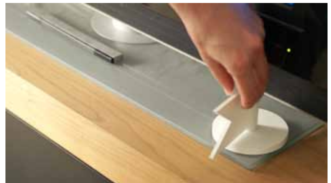
Figure 2 - The Nodes design being used: A user places a node fitted with a receiver (end point of a connection) at the base of a TV.
