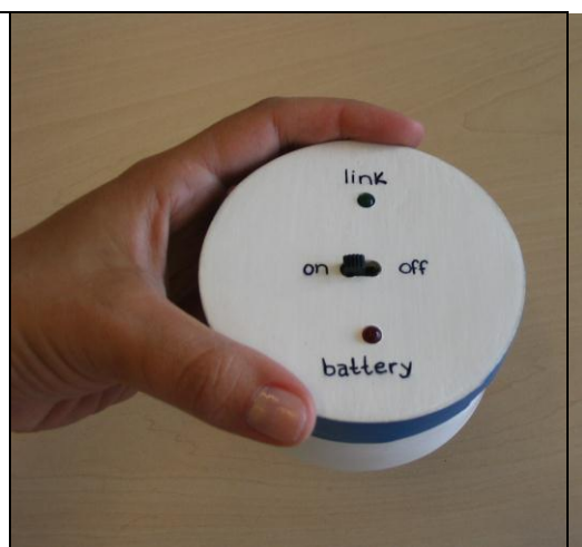
Figure 22. RF transmitter in the second prototype
