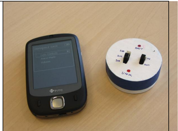
Figure 19. parent's unit (left) and RF transmitter (right) in the first prototype
