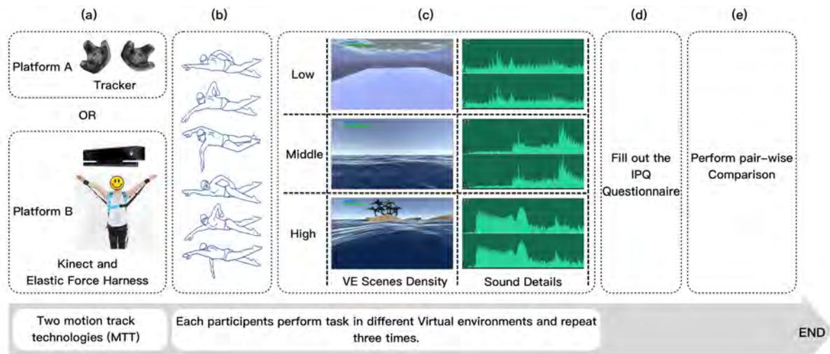
**Figure 8.** Experiment procedure: (a) each participant is provided an instruction manual of using the Swimming Simulator in various MTTs. (b) six components of freestyle stroke practice. (c) Visual scene and sound samples classified into three levels low (low details), middle, and high (high details). (d) participants were invited to fill out the IPQ questionnaire. (e) participants were invited to complete an individual pairwise comparison matrix.
