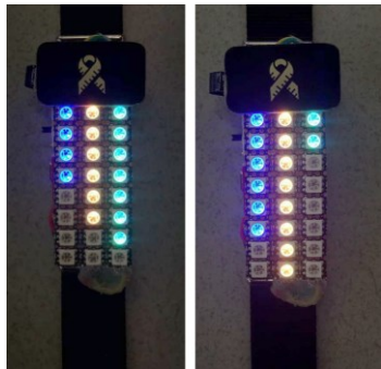
Figure 5: Two examples of the representation of wearer's health-related data through the RGB LED matrix on an i-Ribbon.
