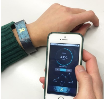
Figure 3: Non-functional mock-up of i-Ribbon made for the early iteration [21].
