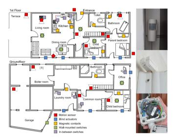
*Figure 1.* Left: Floor plan of the testbed house and sensor placements for the ambient sensor network. Right: Examples of the sensors: a motion sensor on the wall (top), a magnetic contact on a shower door (center), and an in-between switch for the TV (bottom).
