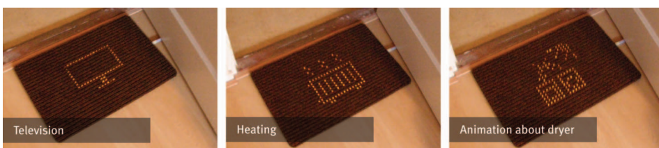
Figure 4. Doormate integrated with a low resolution LED display.
