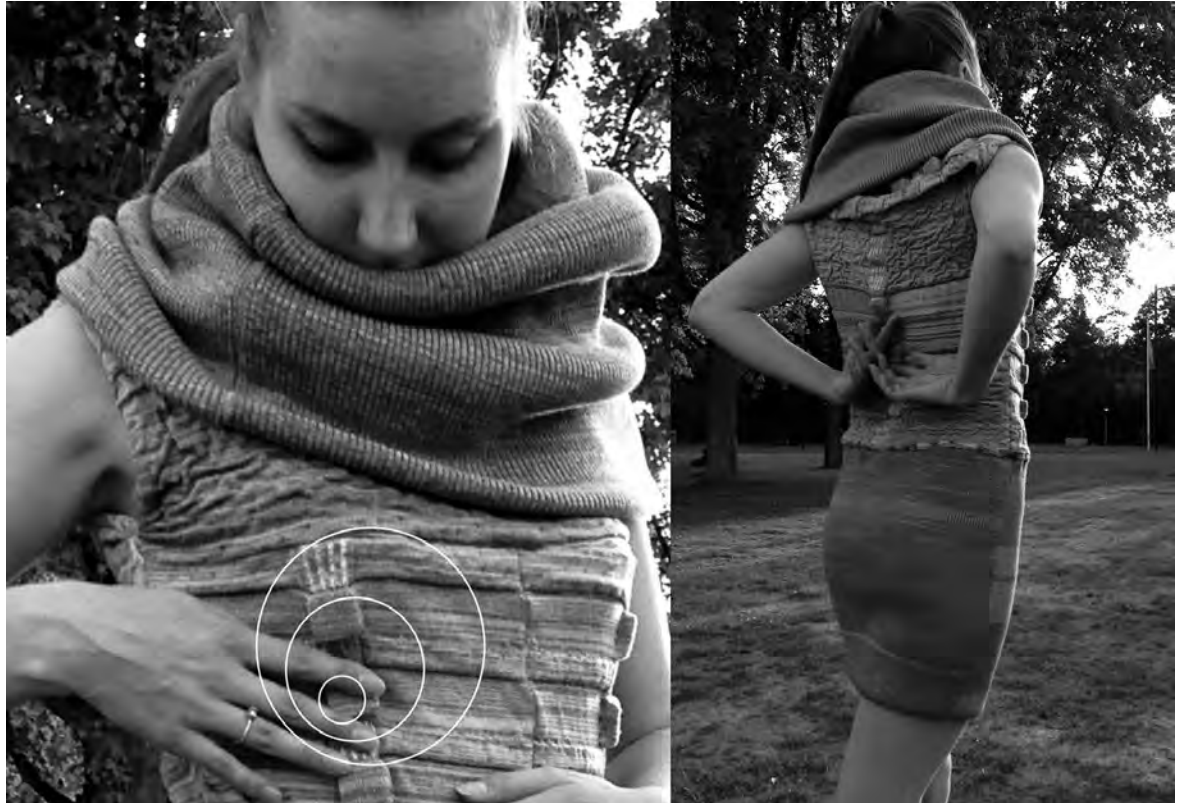
Fig. 1. Left: front of Vibe-ing with two rows of pockets. The white circles visualize the vibration of the modules. Right: back, with the pockets containing the vibration and touch modules on the spine and shoulders. The silver lines are the connection lines between pockets
