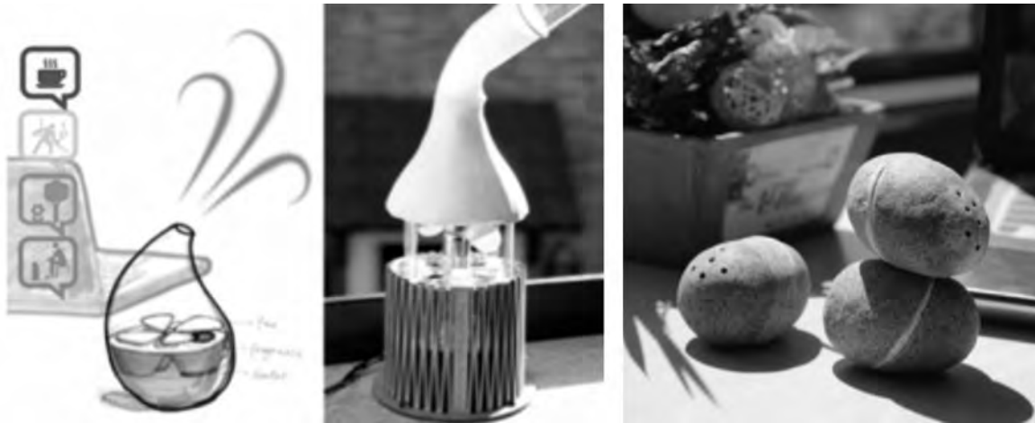
Fig. 6. Example Ambient Experience: Initial concept sketch and prototype (left). Zen Pebble, Intelligent Aroma Diffuser. Emotion detecting software is used to release aroma at an appropriate moment through Zen Pebbles (right) – TU/e student project by Sherry Hui Wang
