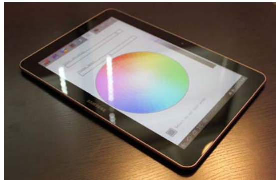
Figure 4. An Android tablet is used to control the dynamic lighting settings from outside the experiment room via a wireless network.
