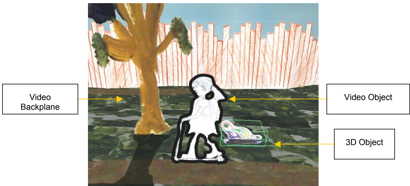
Figure 12: Content production: MPEG-4 scenes composed of different media objects.
